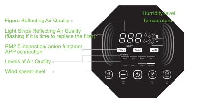
Start Button: When the air purifier is powered up, the "Start button" turns red, and enters the standby mode; press the button to start the machine; the standby-mode power consumption is less than 2W; separate the machine from its source of power to shut it down completely (Note: in the smart mode, anion function runs automatically, and sensor begins to inspect the machine).
